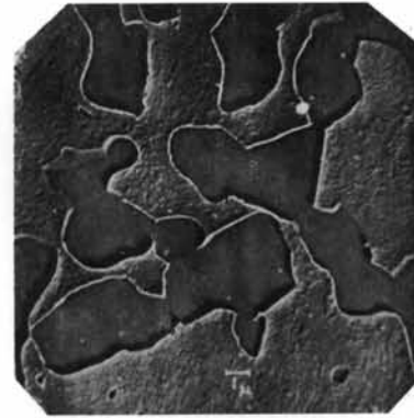
Fig. 6. Electron micrograph of shadowed surface replica from 18/8/Mo/Ti steel after heat treatment for 24 hr. at 850° C. Magnification 2500 \times .
