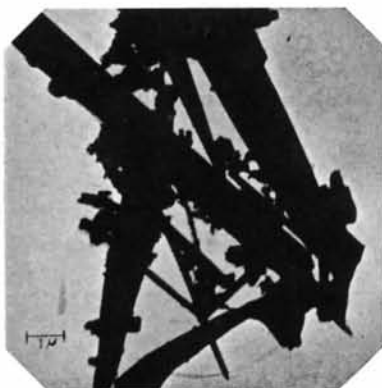
Fig. 7. Electron micrograph of needles of \sigma phase extracted electrolytically from heat-treated 25/20 steel. Magnification 5000 \times .
